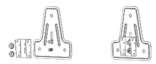
4/ Now position the TOP assemblies on to the top two positions that you marked on the wall and mark these 3 holes for drilling
