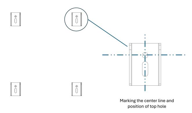
2/ Assemble 2 radiator brackets to the Bullfix Support Brackets in the TOP configuration as shown below
