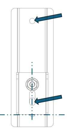
6/ Using a 20mm spade bit drill the 8 holes and insert Bullfix plasterboard fixings as illustrated
