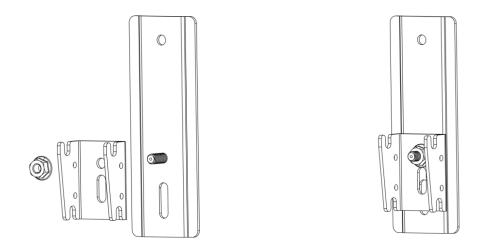
4/ Now position the TOP assemblies on to the top two positions that you marked on the wall and mark these 2 holes for drilling
