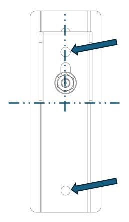
5/ Now position the BOTTOM assemblies on to the bottom two positions that you marked on the wall and mark these 2 holes for drilling
